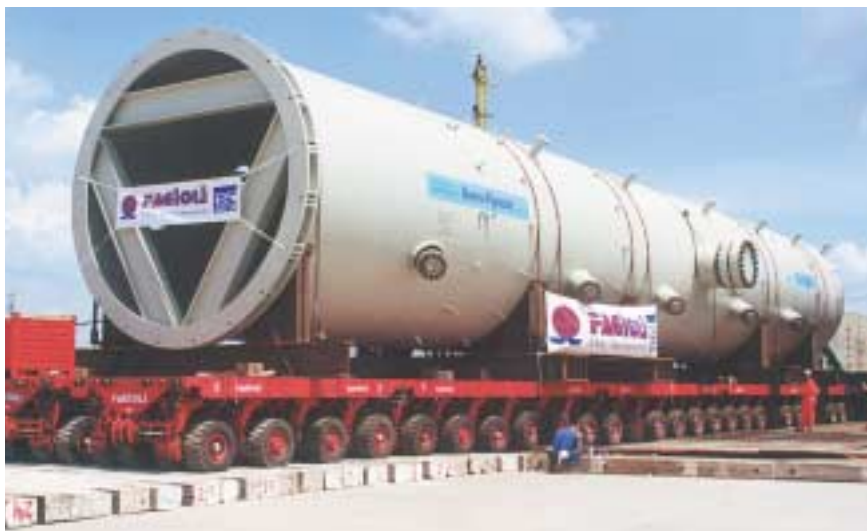
This 1,378-ton hydrocracker reactor, the heaviest piece of equipment ever offloaded at the Port of Beaumont, was discharged from the m.v. Clipper Cheyenne over the port's roll on-roll off ramp.
