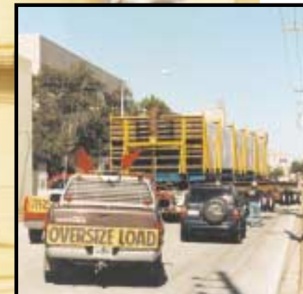
The ‘oversize load’, a module for a heat recovery steam generator bound for the new power plant in Deweyville, moves via heavy duty transport truck from the port through downtown Beaumont.
